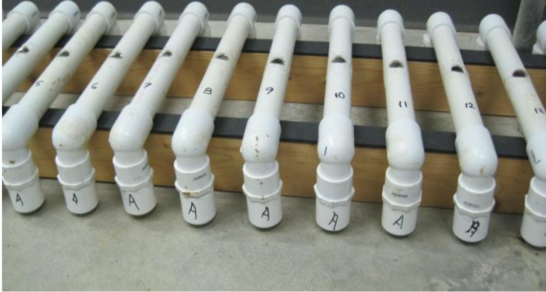
Fig. 3. Horizontal pipes with center hole for introducing grape root borer egg
